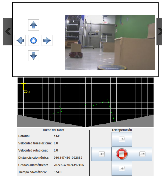
Figure 5. User interface for test scenario 1 with a Pioneer P3-DX robot with ultrasonic sensors and a URG-04LX laser range finder.
