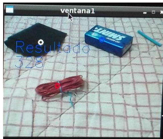
Illustration 5 – Processed Image Proofs with detection of specific colors: black (can-garbage), blue (box-water) and red (cable-inorganic container).
