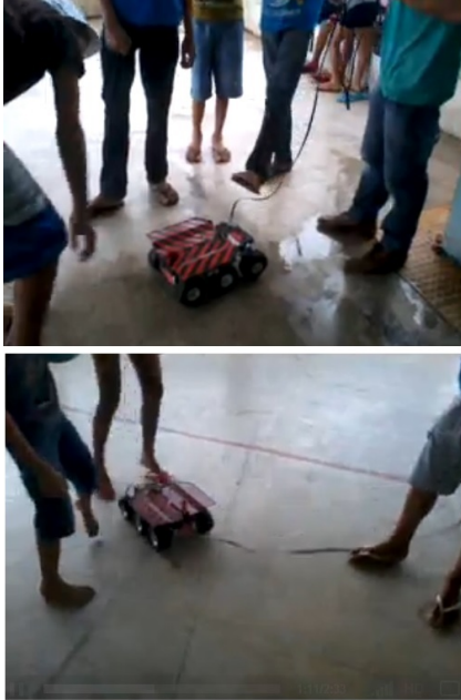
Figura 5: Robot used, testing its obstacle detection in an environment with many people moving.
